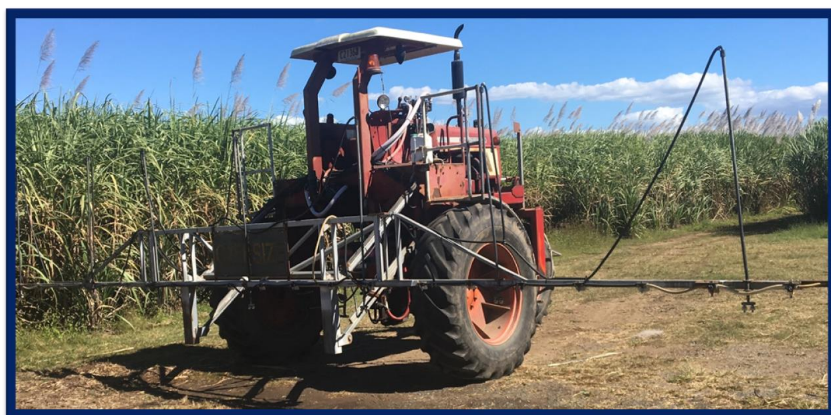
Figure 2- High clearance sprayers provide greater flexibility of product choices and spray timing.
