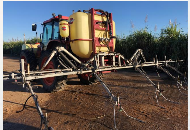
Fig 1. A boom fitted with droppers and Floodjets®
