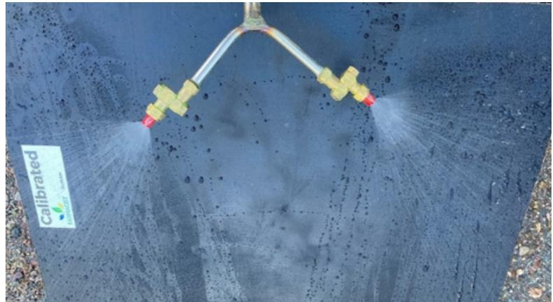
Figure 1 (above): A CFLD-XC 04 nozzle running at 2 bar – extra coarse droplets minimise drift.
