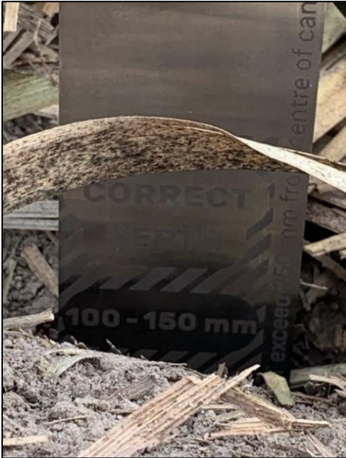
Figure 4- Measuring liquid placement depth is essential.
