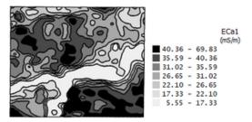
The Topsoil Mapper (TSM) is a precision agronomy tool that utilises electromagnetic induction via soil sensors to create conductivity measurements. The sensor generates data that delineates soil compaction, water content, precise soil zones, and subsoil variance.
